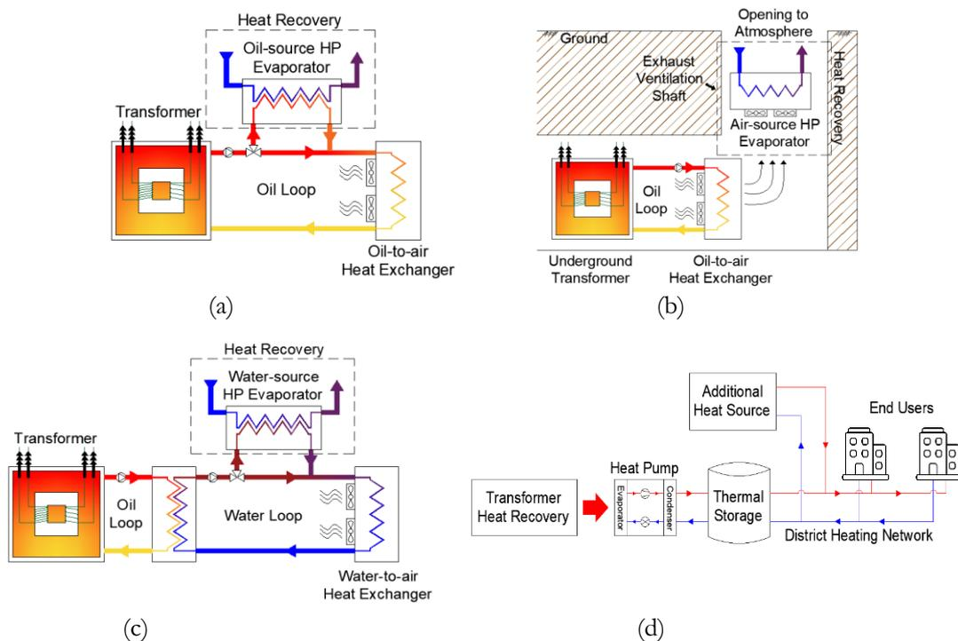
Figure 1 Potential electrical transformer heat recovery options, for: (a) oil forced air forced (OFAF) cooling system; (b) subterranean oil forced air forced (OFAF) cooling system; (c) oil forced water forced (OFWF) cooling system; (d) overall heat delivery system comprising heat recovery, HP, thermal storage and district heating network components.
