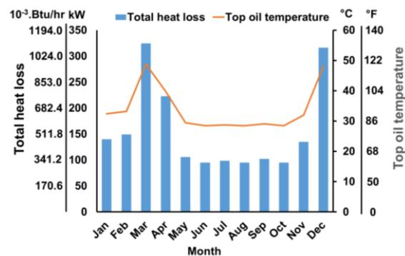
Figure 3 Calculated monthly heat loss rates and top oil temperatures for 90 MVA transformer
