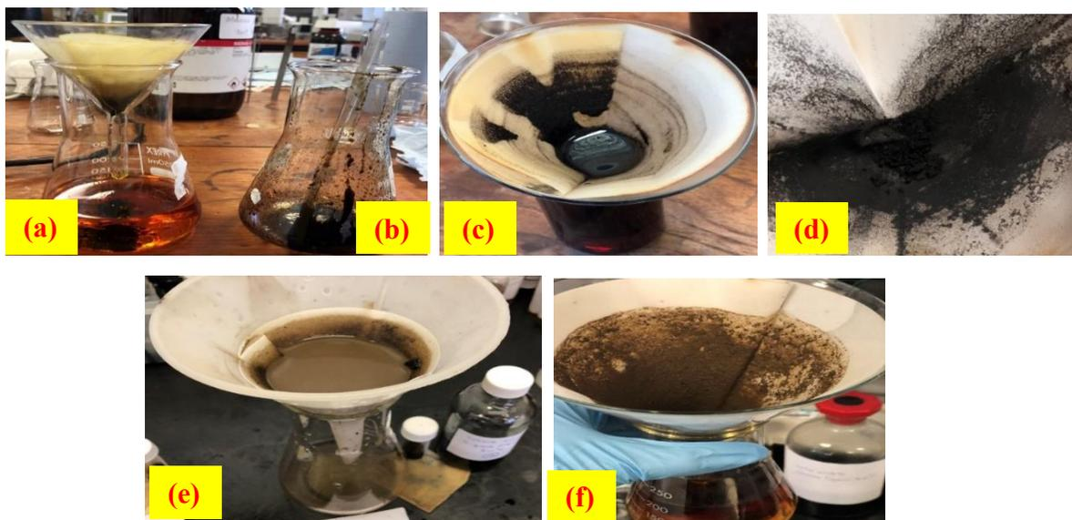
Figure 5. Illustration of bio-oil fractions by (a) toluene soluble, (b) toluene insoluble, (c) methanol soluble, (d) methanol insoluble, (e) water soluble, (f) water insoluble
