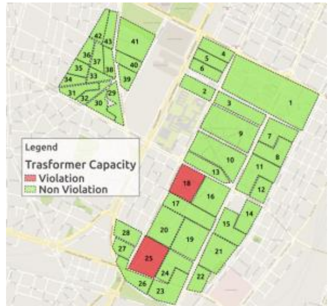
Figure 6. Transformer violation capacity map
