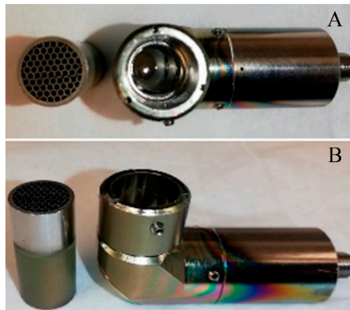
Figure 4. The collimator is fitted with a cylindrical honeycomb filter that prevents coating of the collimator lens. (A): Top view, showing the honeycomb lens protector. (B): Side view.
