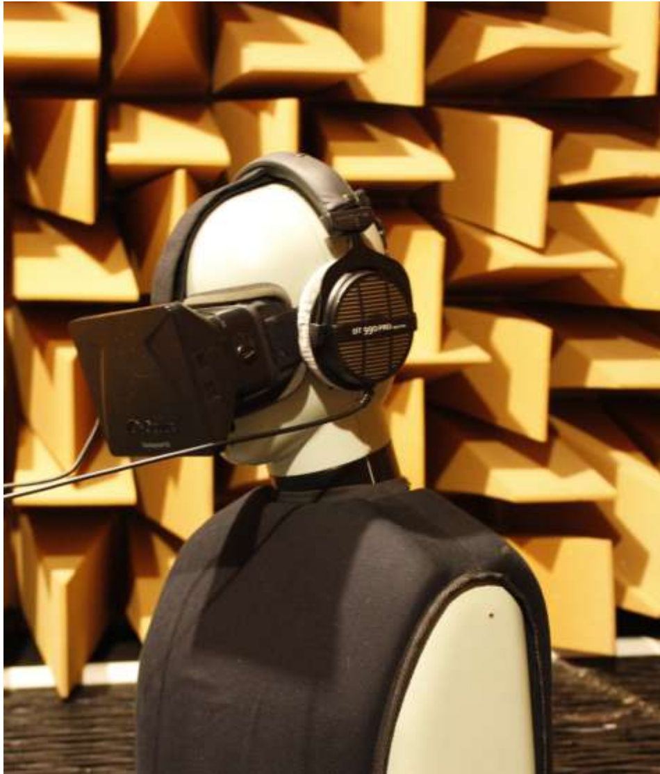
Figure 1: Dummy head equipped with a VR headset display and headphones
