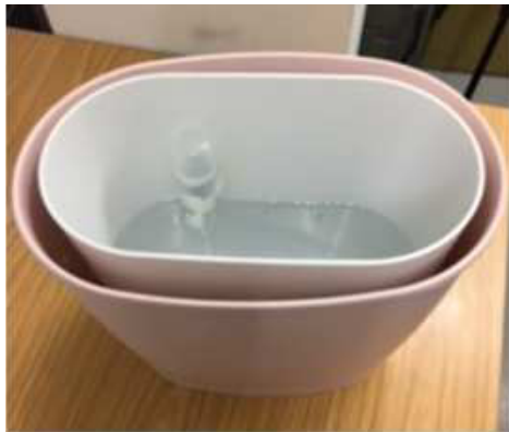
Figure 2: The lung COVID-19 infection fabricated phantom.
