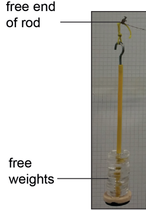
Figure 2.6: Experimental procedure for dead loading. The rod is loaded at the tip with free weights (mass of each is 1.3g).
