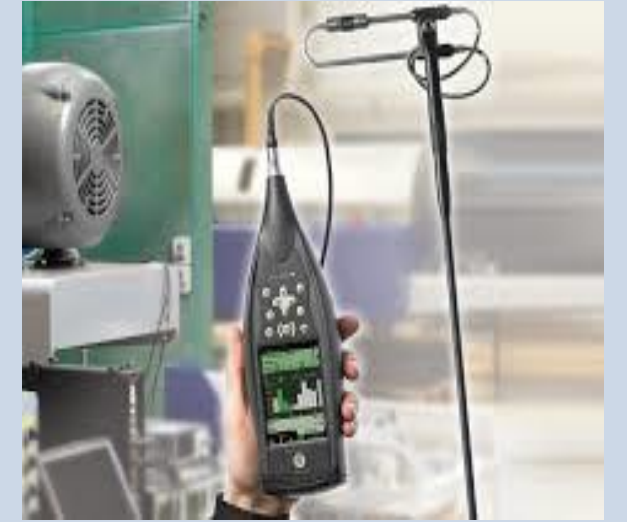
Fig 6. Demonstration of Sound Intensity used for measuring fan's sound power levels, image courtesy of Bruel & Kaejer
