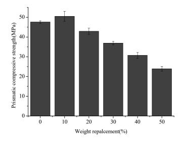
Fig.3. Influence of SSP replacement ratios on prismatic compressive strength 3.2.1.3. The relationship between cubic compressive strength and prismatic compressive strength
