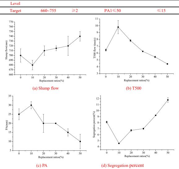
Fig.1. The fresh properties of SCRAC with SSP at different replacement ratios
