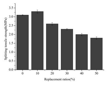
Fig.5. The splitting tensile strength for various samples.
