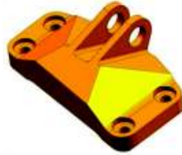
Figure 1: Original Design Envelope for Engine Bracket [1]
