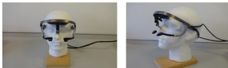
2239 Figure 9. Head mounted eye tracker which was worn like glasses.
