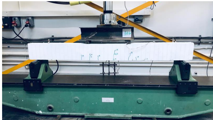
Figure 5: An image of a beam being tested under four point loading.
