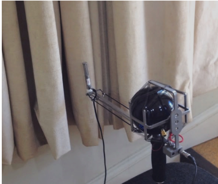
Figure 54: The absorption of the curtains in Henry Wood Hall being measured in-situ with the Microflow Impedance Gun [160].
