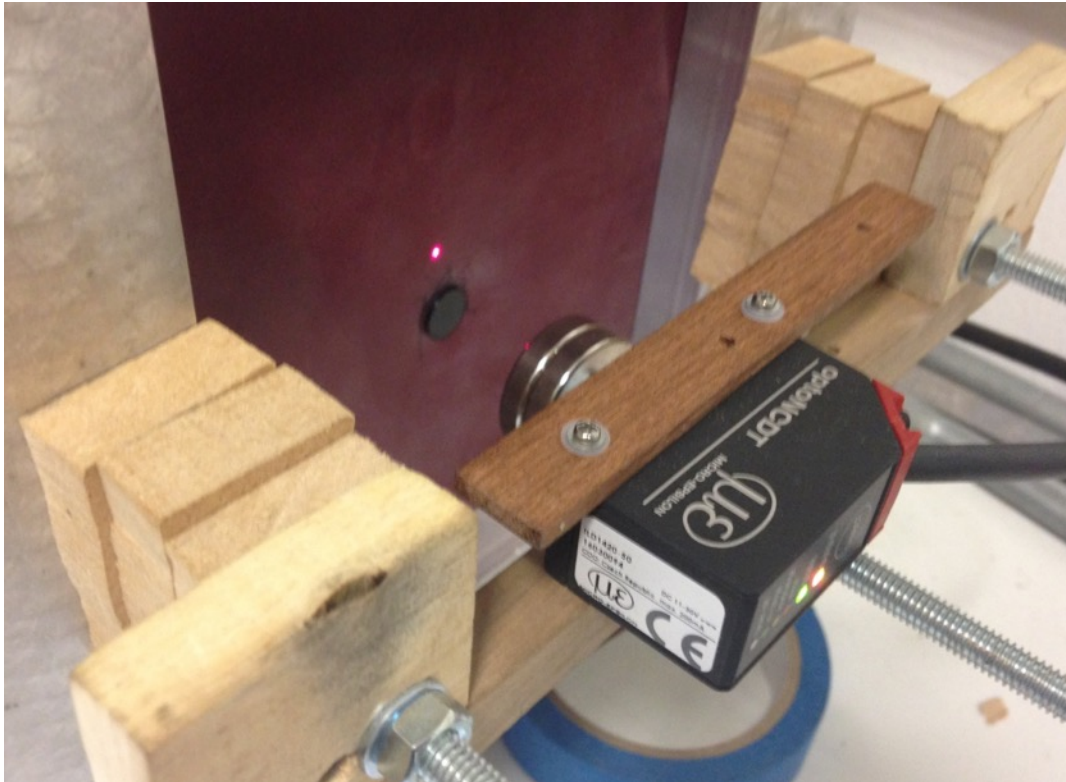
Figure 95: First pilot test of single magnet embedded in membrane, attracted by single permanent magnet. The latter was replaced by a toroidal electromagnet for measurements.
