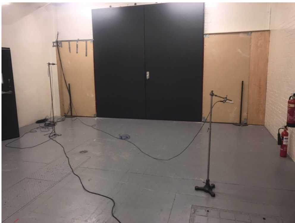
Figure 35: False walls constructed in LSBU reverberation chamber. In “closed” condition
