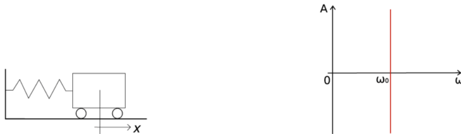
Figure 18: Linear oscillator, frequency does not depend on amplitude; the resonant frequency \omega_0 is unchanged by system amplitude. (From Bellet [120]. Reproduced with permission).
