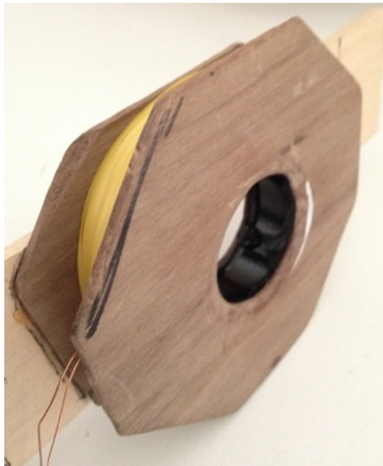
Figure 97: Simple electromagnet constructed for tests.
