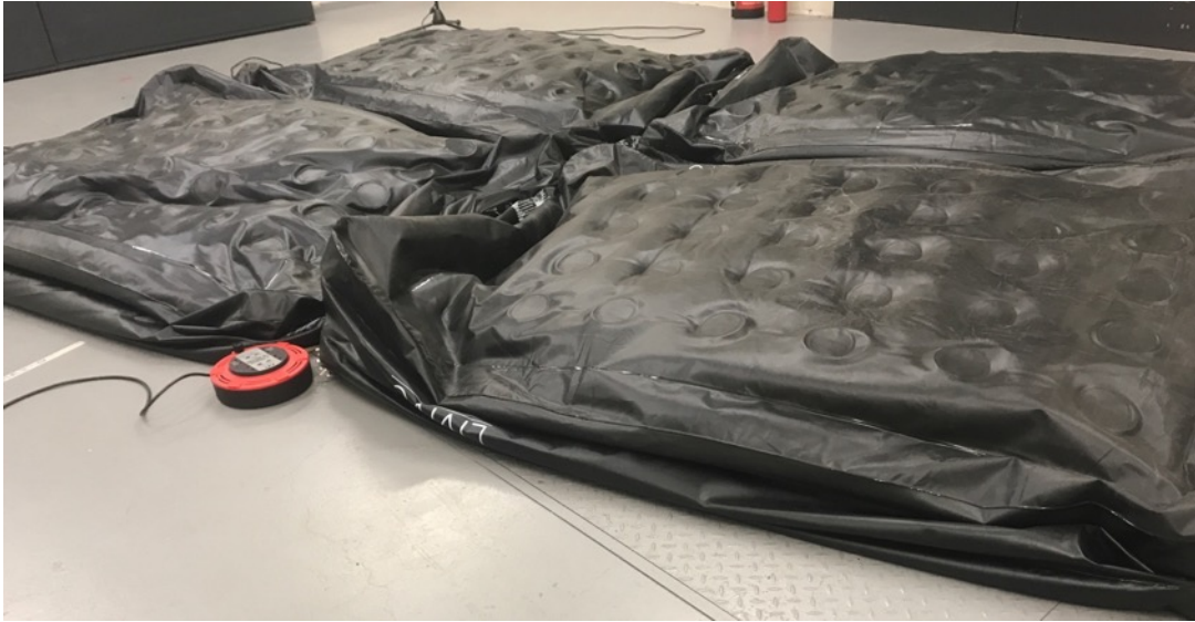
Figure 64: Partially inflated airbeds during inflation tests.
