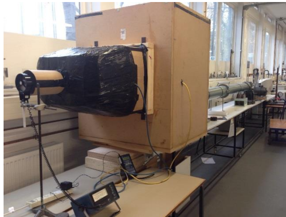
Figure 4.1 Air flow test rig with the enclosure with resonators and adaptor applied to it.
