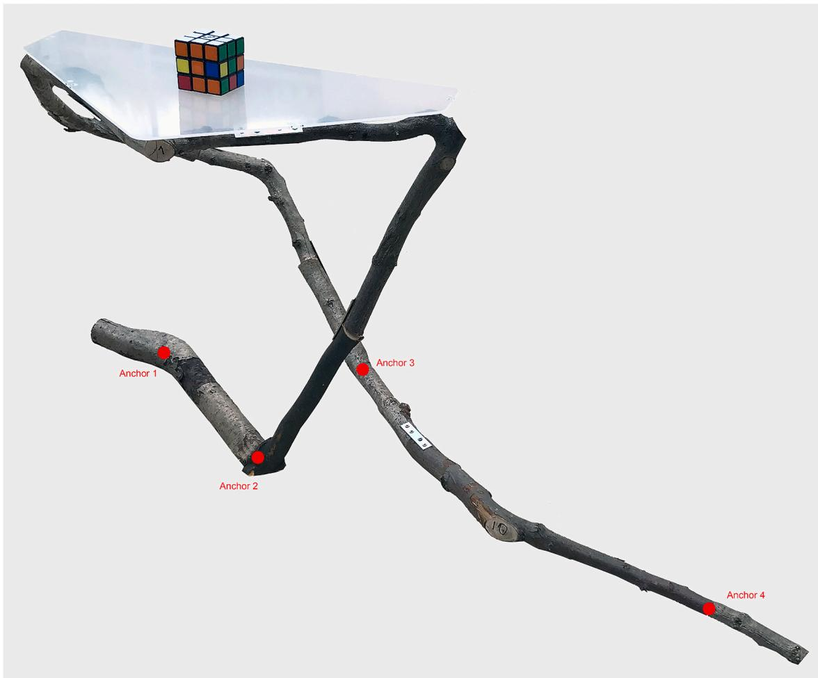
Fig. 19. Fabricated table with ten tree forks collected from a forest, put together based on the instructions generated by the GA.
