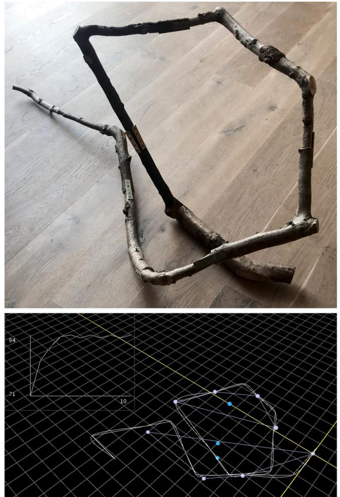
Fig. 17. Fabricated table with ten tree forks collected from a forest, put together based on the instructions generated by the GA.
