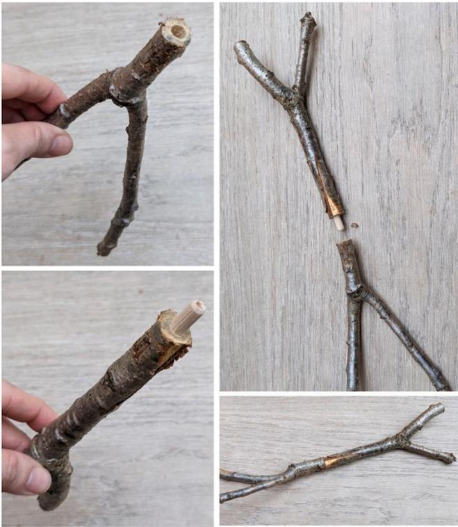
Fig. 16. Wooden dowel joint experiment on two thin tree forks.
