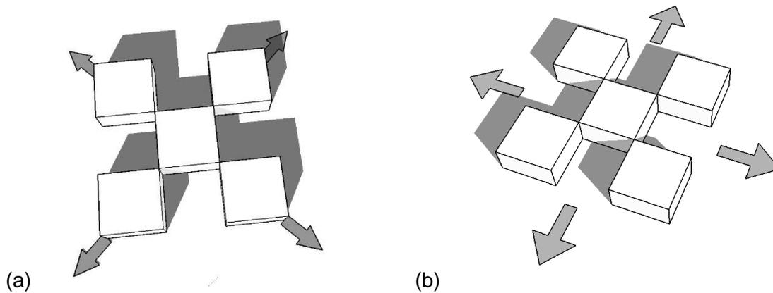
Fig 2.0 (a) Cross-vault pixelation showing the direction of lateral forces. (b) Pyramid pixelation showing the result of outward expansion (Source: Authors)
