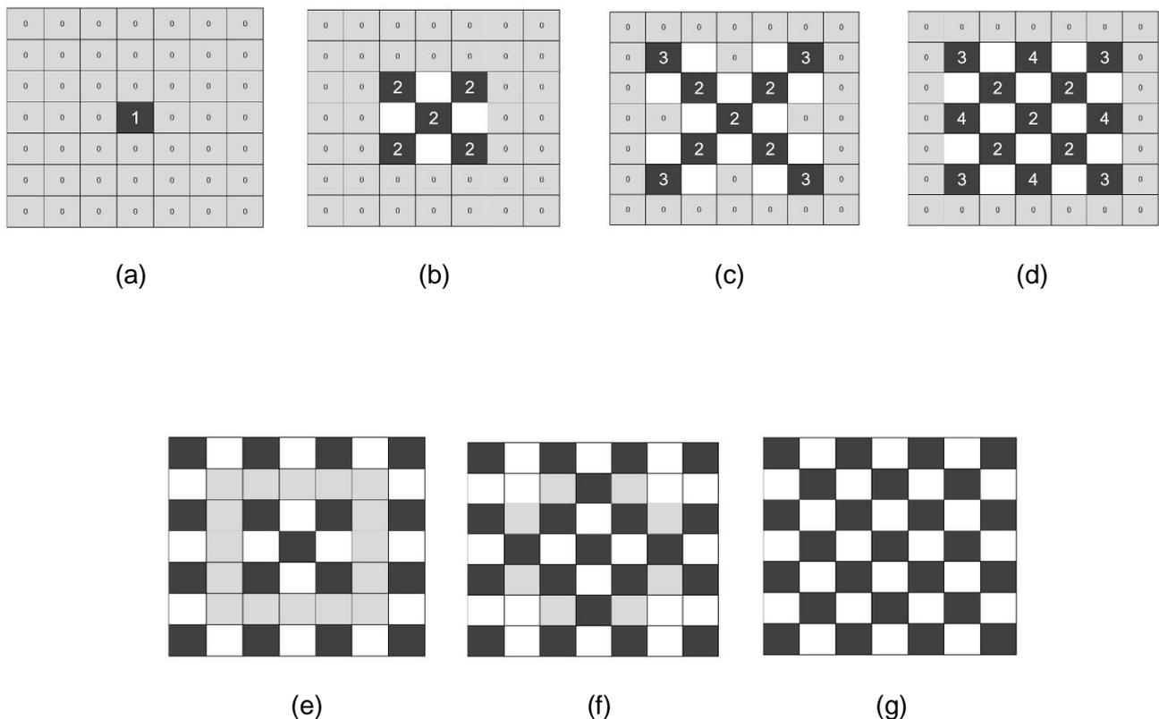
Fig. 8.0 (a) (First step)= $x=1$  (b) Second Step= $x=2$ ,  $y$ =(No. of blocks)=5 (c)  $x=3$ ,  $y=9$  (d)  $x=4$ ,  $y=13$  (e)  $x=5$ ,  $y=17$  (f) (6,21) (g) (7,25) (Source: Authors)
