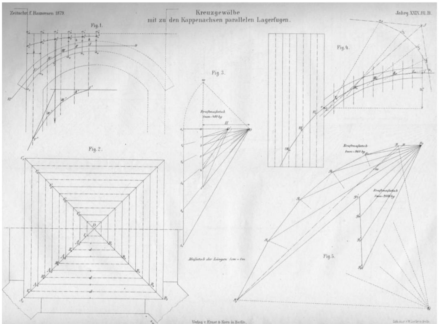
Fig. 7.0 The first known application of thrust-line analysis combined with the slicing technique by Wittmann (1879)
