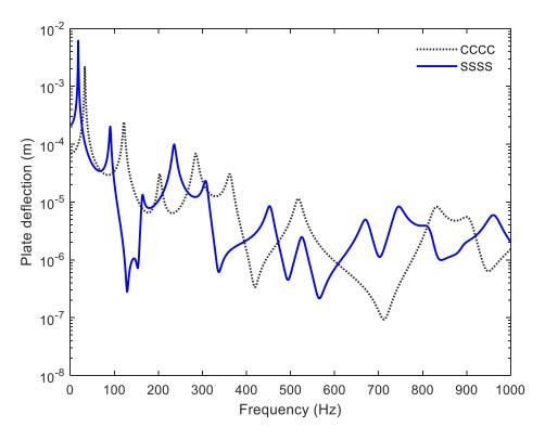
Figure 3: Deflection of simply supported and clamped fibreglass plate at x = 0.15 m and y = 0.15 m
