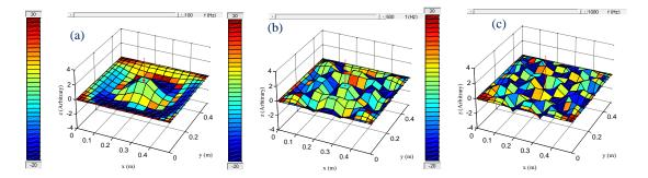
Figure 5: 3D deformation of fibreglass composite clamped plate at a) 100 Hz, b) 500 Hz, and c) 1 kHz respectively.
