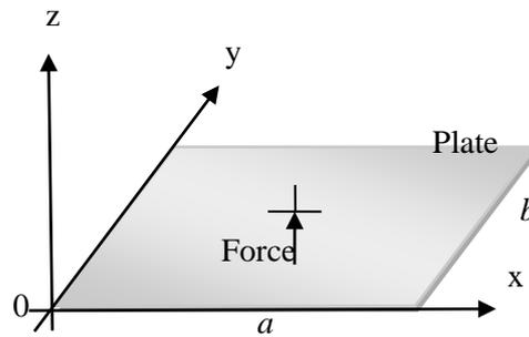
Figure 1: The geometry of a baffled plate.
