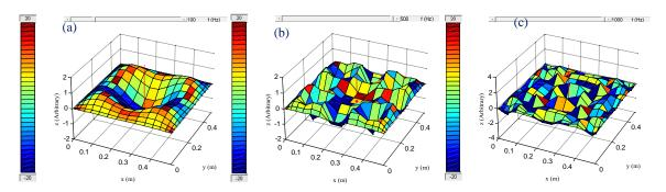
Figure 4: 3D deformation of fibreglass composite simply supported plate at a) 100 Hz, b) 500 Hz, and c) 1 kHz.
