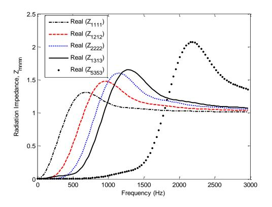
Figure 6: Radiation impedance matrix, direct terms.
