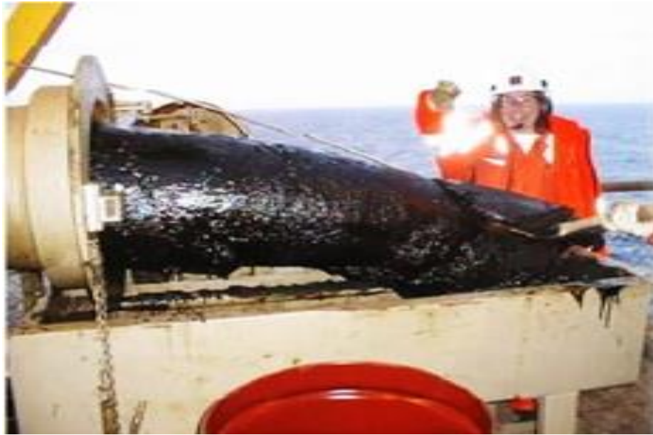
Figure 1: Wax deposition plug in the wellbore on platform C in the North Sea (Akpabio, 2013).
