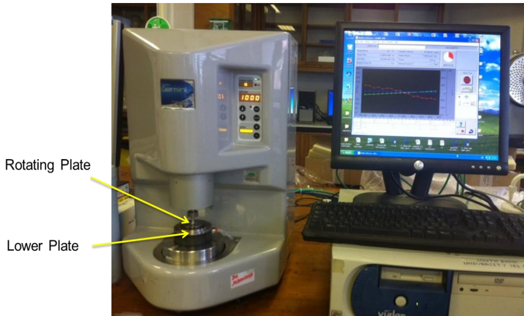
Figure 15: A Bohlin Gemini II Rheometer used to measure WAT (LSBU).
