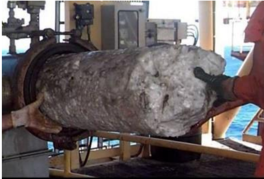
Figure 2: Hydrate plug formed in a subsea hydrocarbon pipeline (Irmann-Jacobsen, 2013; Heriot-Watt University, 2014).
