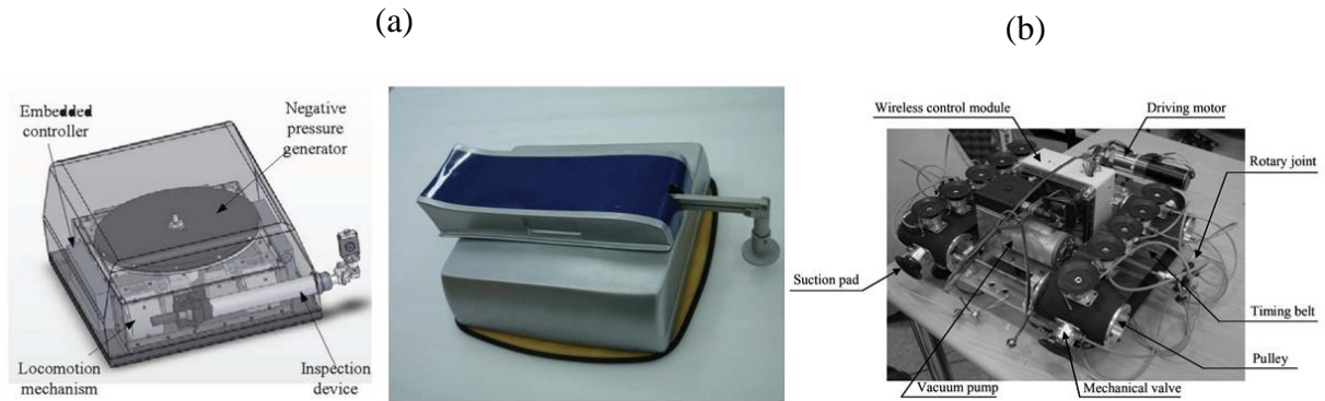
Figure 2-15: (a) Vortex-type suction mechanism assisted robot [77]; (b) suction cups – tracked crawler robot [151]
