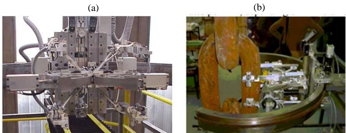
Figure 2-3: Automated weld inspection mechanism [23]. (a) Prototyped version. (b) testing
