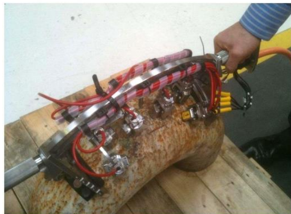
Figure 6-6: TWI's handheld chain crown inspection device [119]
