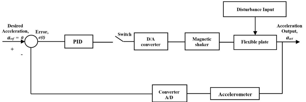
**Figure 20:** The schematic diagram of the controller used in the experiment
