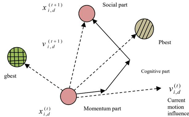
**Figure 10:** description of velocity and position updates in PSO for a two dimensional parameter space
