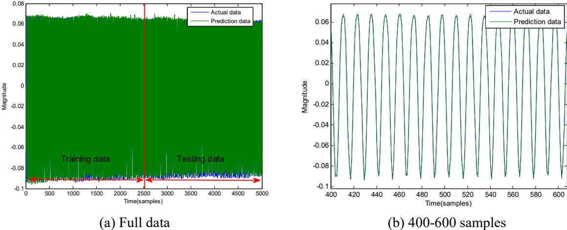
Figure 4: System output in time domain using PSO modeling
