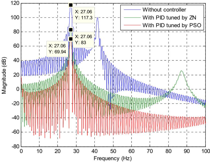
Figure 13: PID controller tuned by ZN and PSO methods for vibration suppression in frequency domain using multiple sinusoidal disturbance
