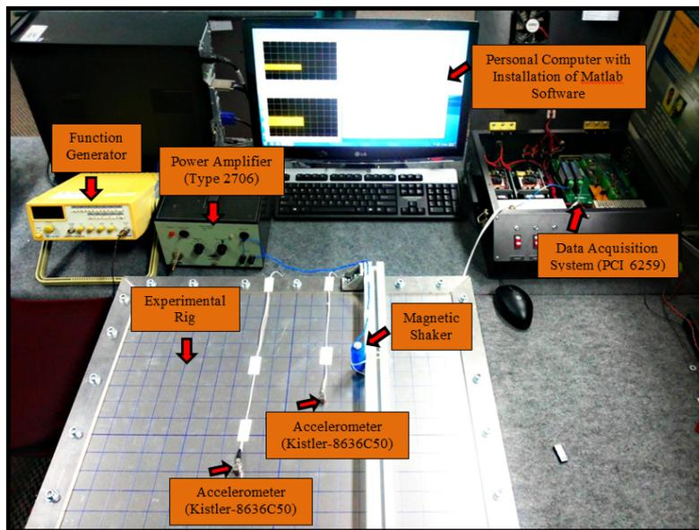
**Figure 1:** The experimental setup for collecting input-output vibration data.
