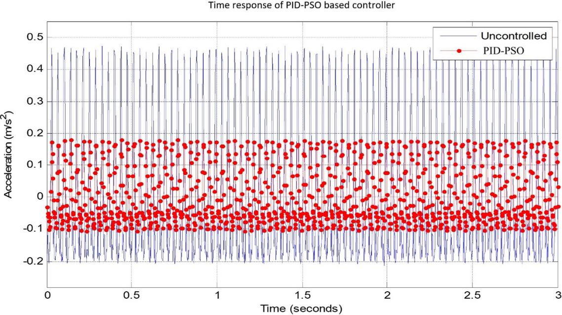
Figure 22: Experimental time response of PID based controller tuned by PSO algorithm
