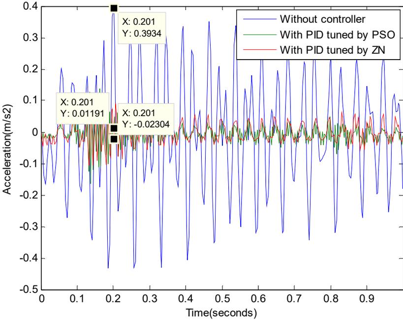
Figure 16: PID controller tuned by ZN and PSO methods for vibration suppression in time domain using multiple real disturbance.
