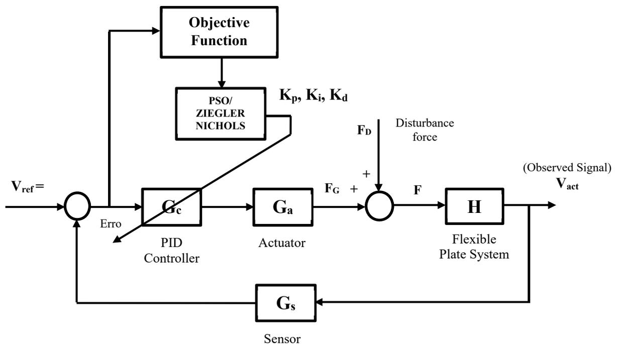
**Figure 9:** The block diagram of PID based controller tuned by Ziegler-Nichols and particle swarm optimization methods.
