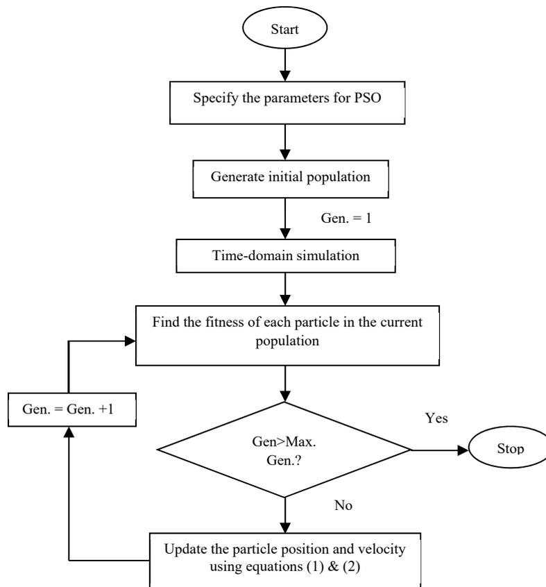
**Figure 11:** The computational flowchart of PSO algorithm
