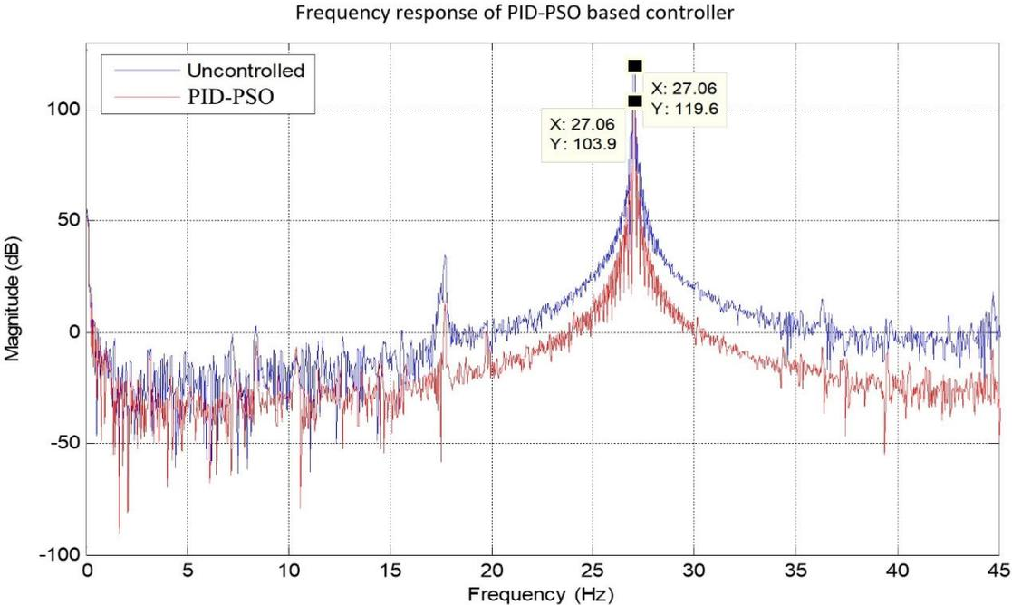
Figure 23: Experimental frequency response of PID based controller tuned by PSO algorithm
