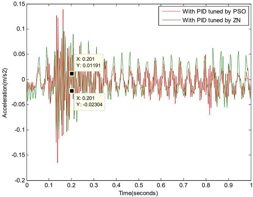
Figure 18: Comparison in time domain between PID-ZN controller and PID-ABC controller with multiple real disturbance.
