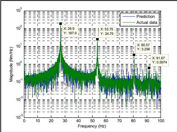
Figure 5: Output and estimated output of the system in Frequency domain using PSO modeling
