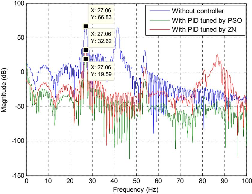
Figure 17: PID controller tuned by ZN and PSO methods for vibration suppression in frequency domain using multiple real disturbance.
