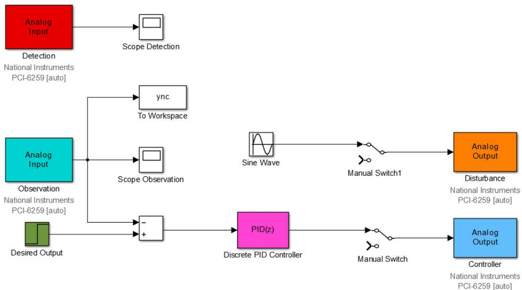
**Figure 21:** Block diagram of PID based controller using MATLAB/Simulink
