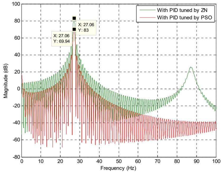
**Figure 15:** Comparison in frequency domain between PID-ZN controller and PID-ABC controller with multiple sinusoidal disturbance
