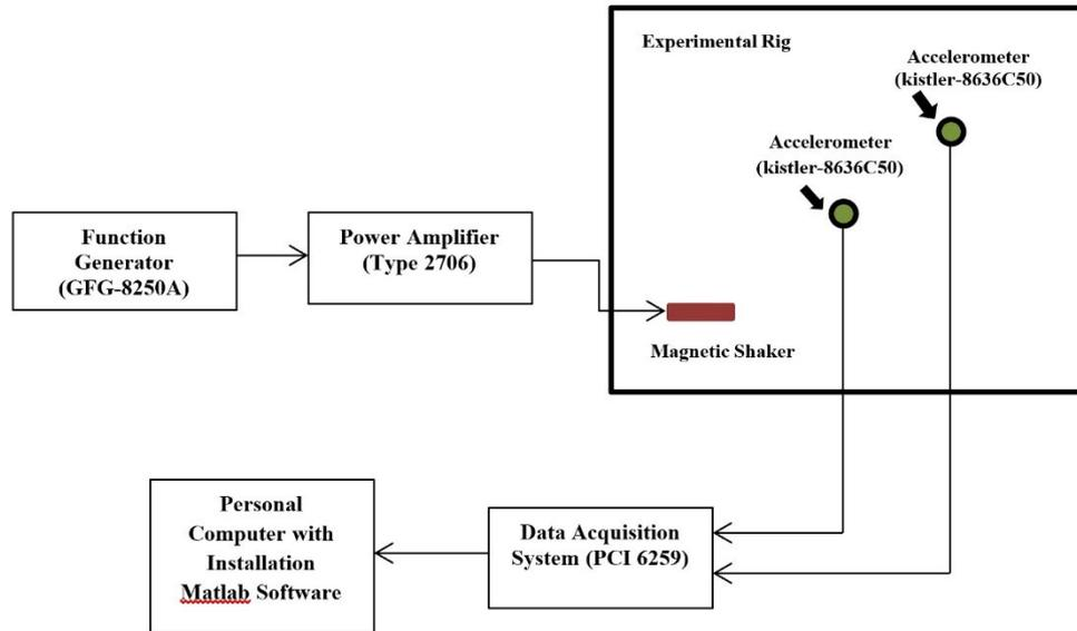
**Figure 2:** The layout of experimental setup
