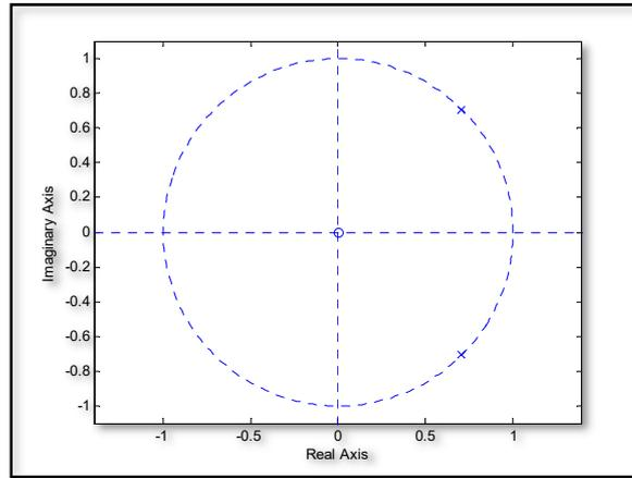
**Figure 7:** Pole-zero diagram of the system using PSO modeling
