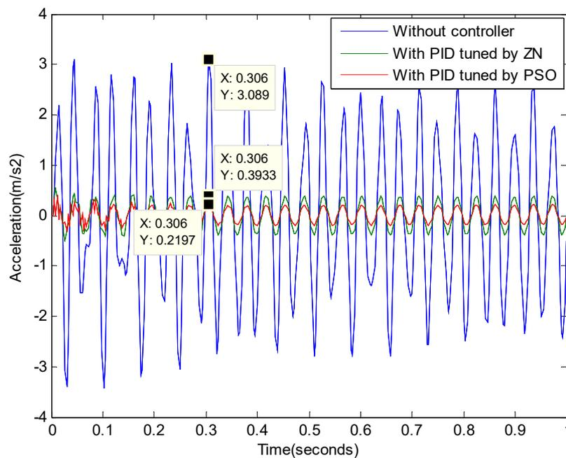
**Figure 12:** PID controller tuned by ZN and PSO methods for vibration suppression in time domain using multiple sinusoidal disturbance
