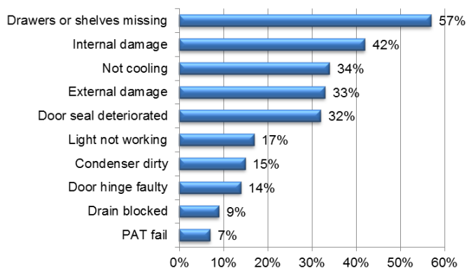
Figure 2. Reasons for failure.
