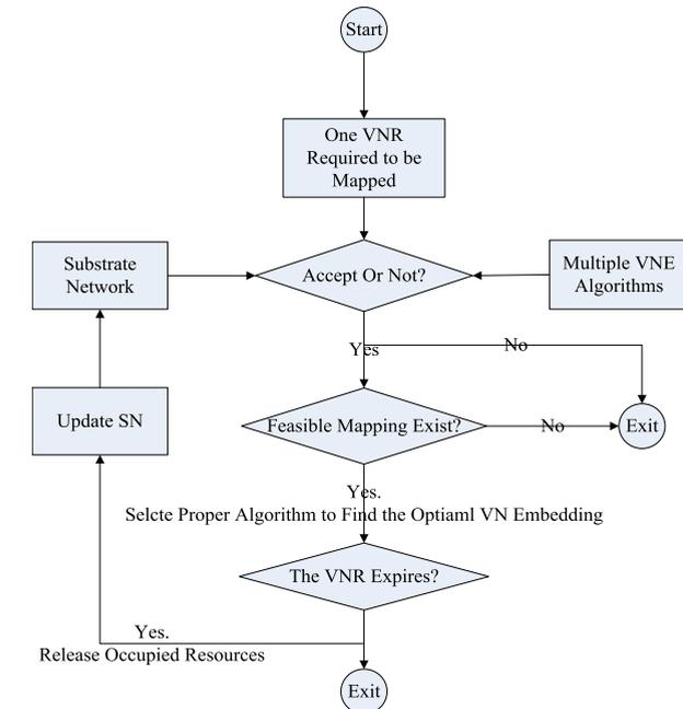
FIGURE 2. Diagram of embedding of one VNR.
