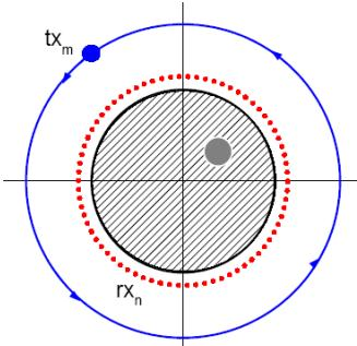
Fig. 1: (color online). Schematic illustration of a section of the system. Transmitting (light blue line) and receiving positions (red dots) containing the sample (black line) are shown. A section of the inclusion (grey circle) is shown inside the receiving circle.
