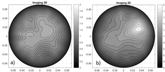
Fig. 3: Images resulting from the analysis. Black and white maps show the dielectrics inhomogeneities (in arbitrary units) reconstructed by Huygens Principle. In order to compare different samples, images have been normalized to the average value to have the same intensity scales. (a) Image relative to the homogeneous oil sample. (b) Image of oil sample having glycol test tube: the white spot highlights the presence of the inclusion. Axis units are in meters [m],
