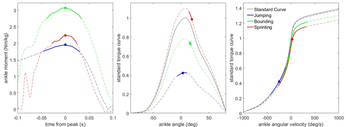
**Figure 1:** An example of the peak ankle joint moments (left), angle (middle), and angular velocity (right) during sprinting (red), bounding (green) and jumping (blue). The standard curve shows the maximum torque available at the optimum angle during isometric conditions.
