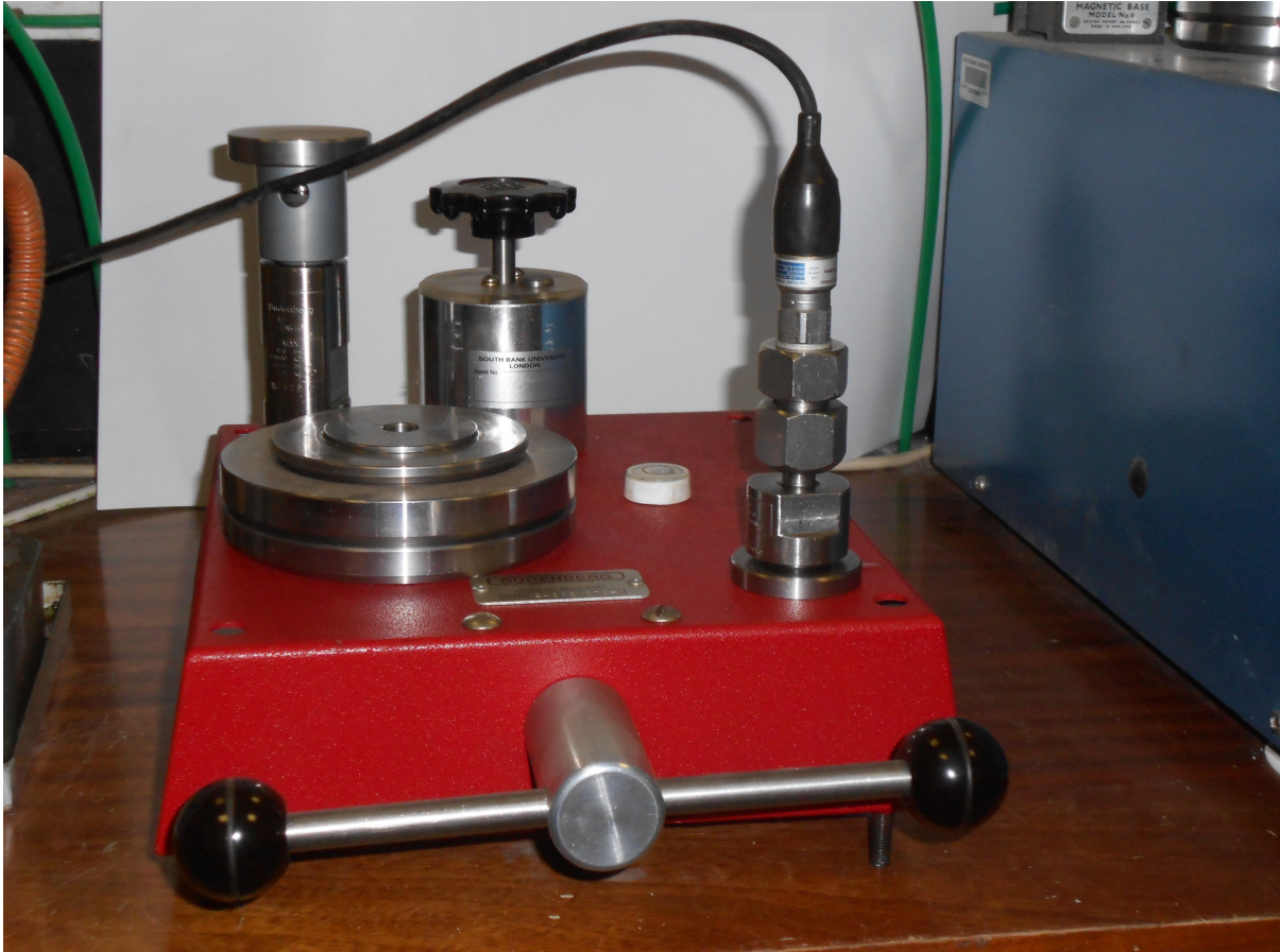
Figure 3.11: Budenburg dead weight calibration unit
