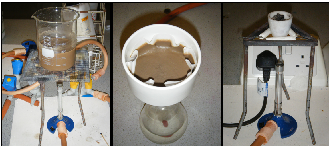
Figure 4.1: Determination of sulphate content on prepared solution – Gravimetric method
