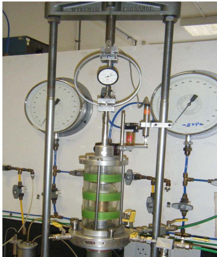
Figure 3.9: Load cell calibration using (WF) body frame and a proving ring
