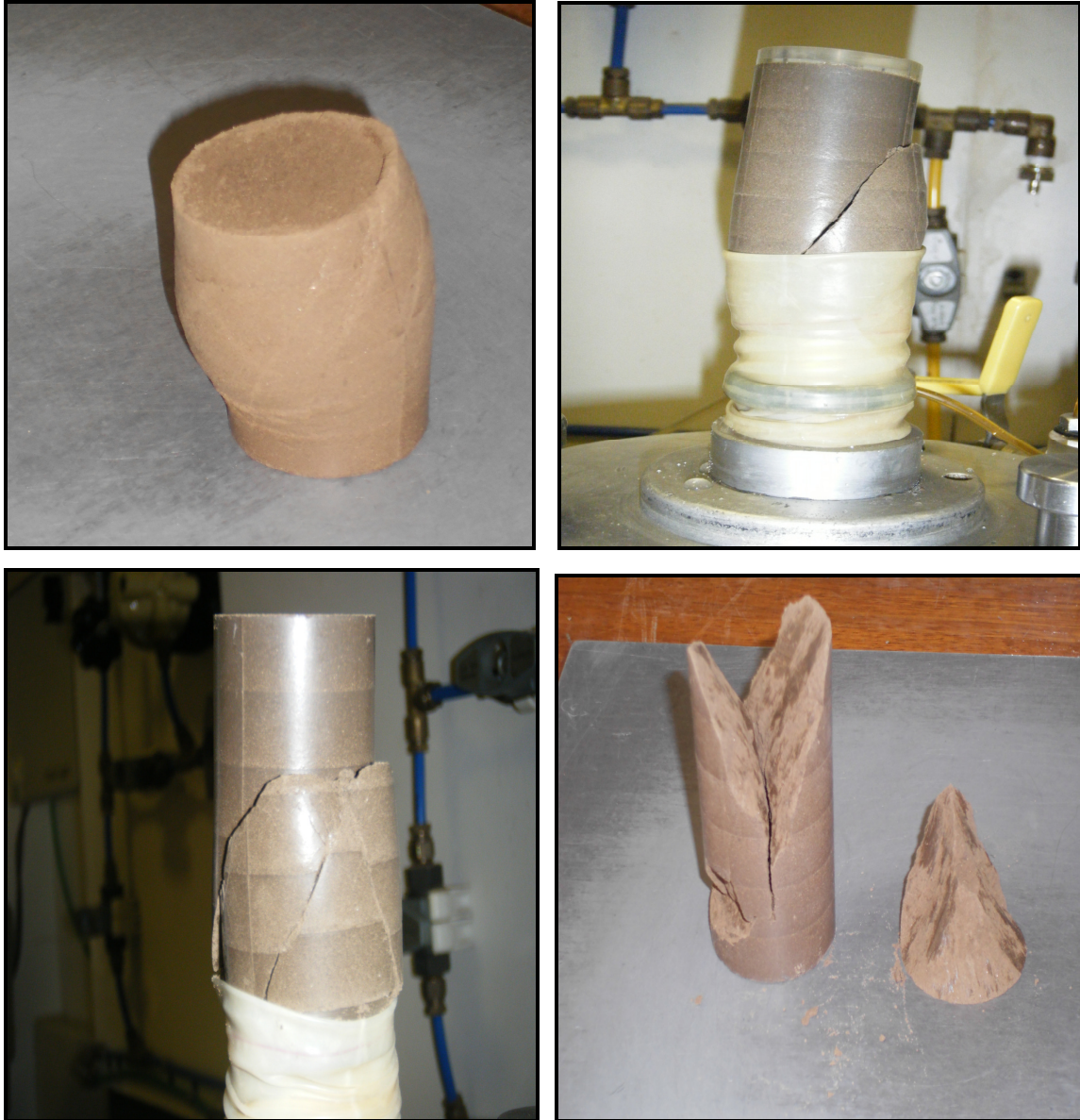
Figure 5.2: Failure type of untreated and lime treated London Clay samples in UU Triaxial tests (Sheared as cured)
