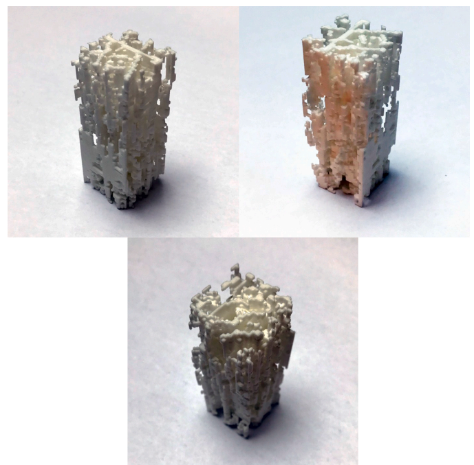
Fig. 27. The 3D printed model of the generated leaf block is stable and stands on its own.
