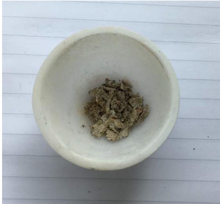
20g Peat sample with 91.8309 % organic contents after combustion in muffle furnace
