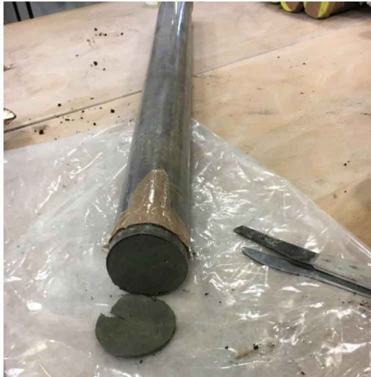
Clay sample from WS02 (5 m depth) with organic content 16.4302 %
