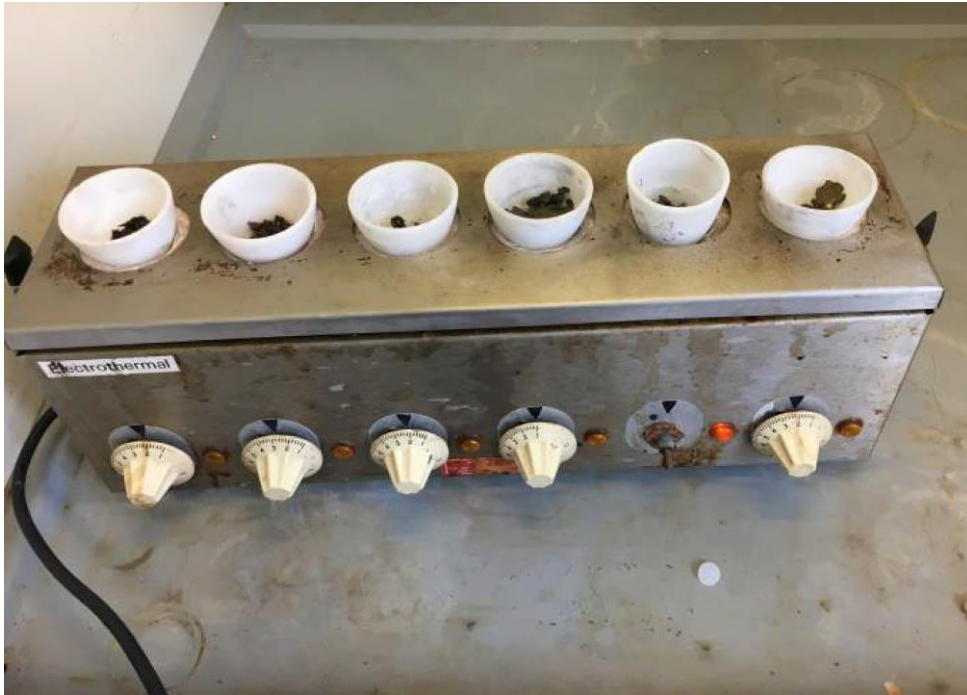
Soil Samples placed on Electrothermal Isomental for preheating, prior to determination of organic contents,
