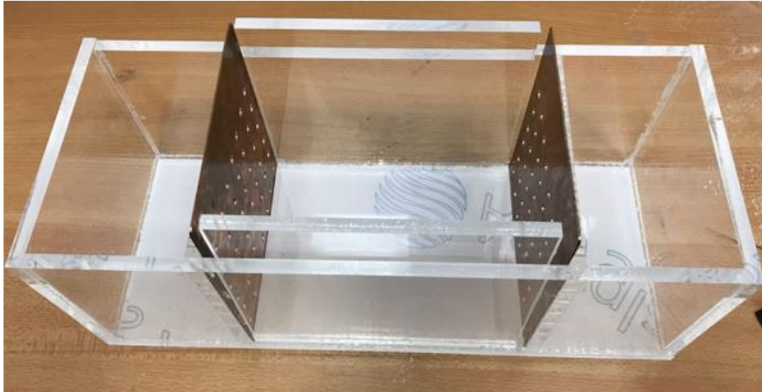
Figure 3.9 Sample extractor and electrode arrangement
