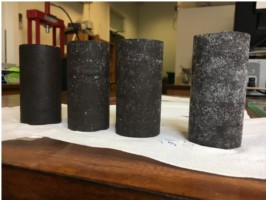
Soil Samples with different % of induced calcite precipitation
