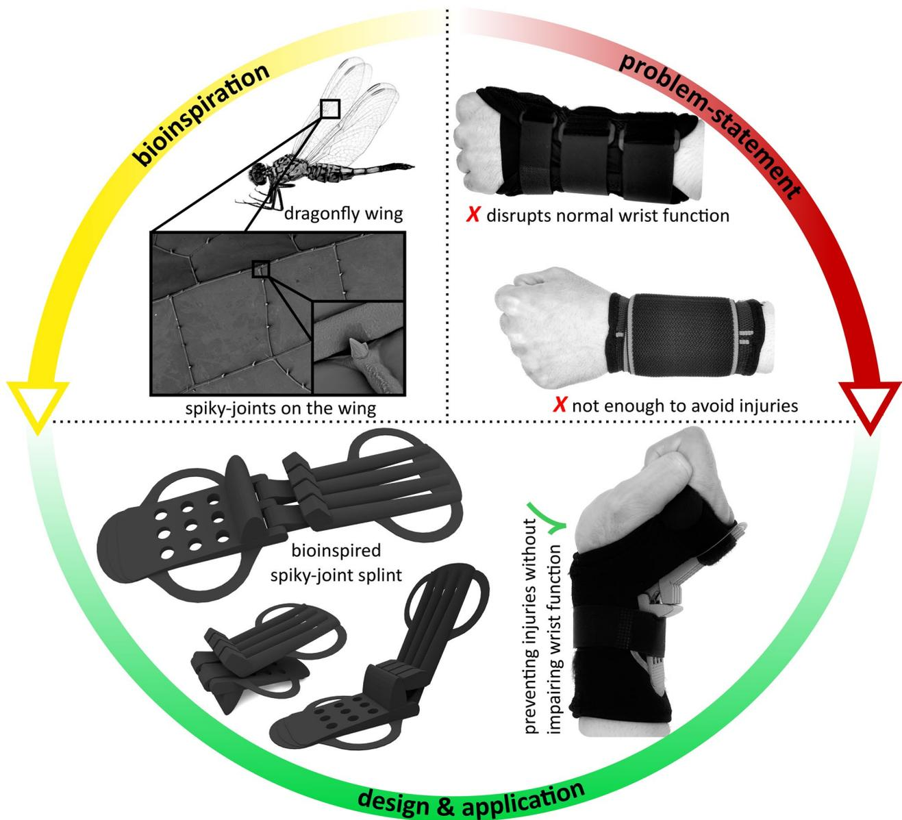
**Keywords** 3D printing · Hyperextension · Wrist support · Wearable device · Orthotic
