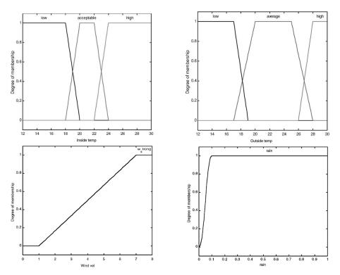
**Figure 4.** Membership function describing inside temperature (**top left**), outside temperature (**top right**), wind velocity (**bottom left**), and rain (**bottom right**) [57].
