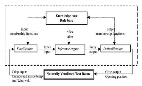
Figure 3. Basic configuration of fuzzy logic controller [57].
