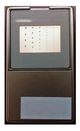
Figure 3.1a Participants' view of the TRU, a new device for measuring amplitude of accommodation
