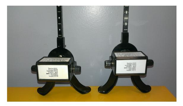
Figure 2.1 Two RAF Rules, showing position of scale differs
