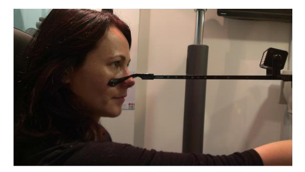
Figure 2.2 RAF Rules in normal use, showing error due to declination
