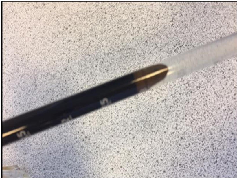
Figure 4-14 Tilted pipette showing non-viscous microemulsion phase formed.
