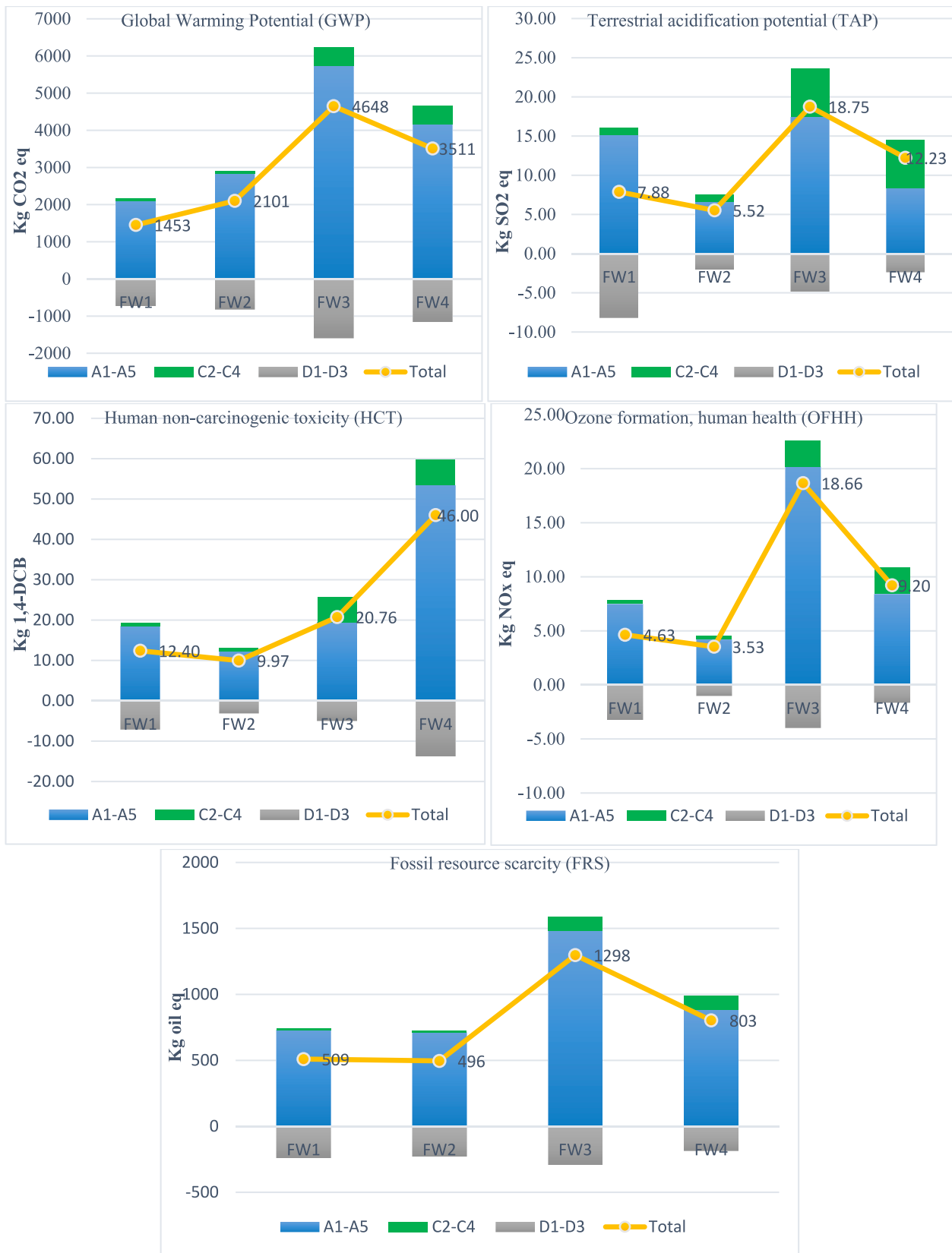
Fig. 4. Life cycle assessment for 50 cycle reuses of formwork, Plastic (FW1), steel (FW2), Plywood (FW3), timber (FW4).
