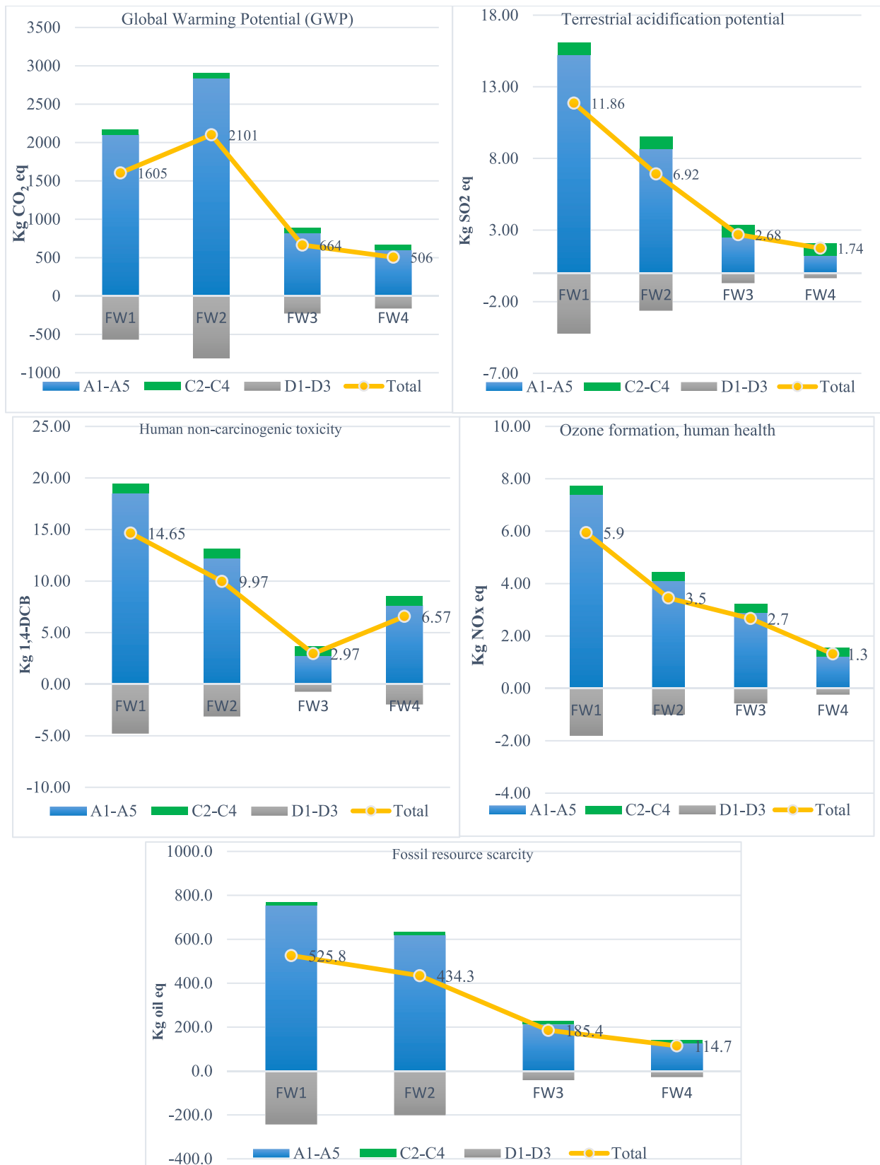
Fig. 3. Life cycle assessment for one cycle of formwork, Plastic (FW1), steel (FW2), Plywood (FW3), timber (FW4).
