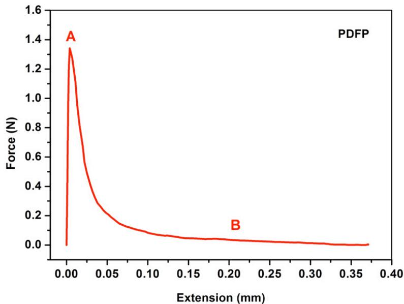
Fig. 3 - Typical force-extension curve recorded during the separation of two PMMA plates adhered together by PDFP.
