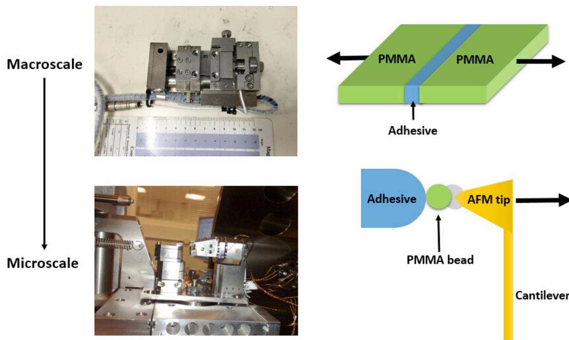
Fig. 1 - Schematic showing the macroscale and microscale tests performed to evaluate the performance of PDFP/PDAC adhesives using (top) a commercial microtester and (bottom) an AFM setup.
