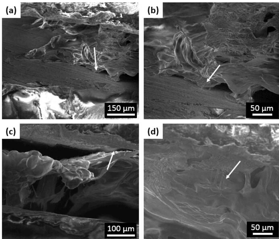
Fig. 4 - Scanning electron micrographs of the PDFP-bonded interface at the yielding point. The images are obtained from different samples and show the delamination behaviour of the PDFP adhesive, indicated by white arrows.
