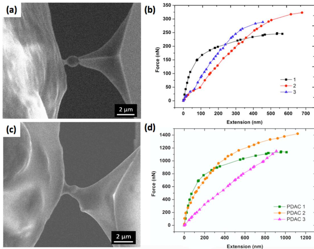
Fig. 9 - (a) Scanning electron micrograph showing the PMMA-coated bead detached from the PDFP adhesive by the Attocube AFM. (b) Force-extension curves of three successful tests on PDFP. (c) SEM micrograph showing a PMMA-coated bead detached from PDAC adhesive. (d) Corresponding force-extension curves for AFM mechanical tests on PDAC.
