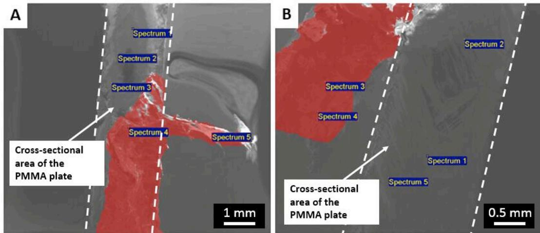
Fig. 6 - SEM images of the cross-sectional area of the PMMA plate with the failed interface of adhesives stretched to extensions A and B in Fig. 5. For both samples, EDS measurements were performed at 5 different locations to probe the chemical composition of the structures imaged, with the red areas indicating the region covered with PDFP adhesive.
