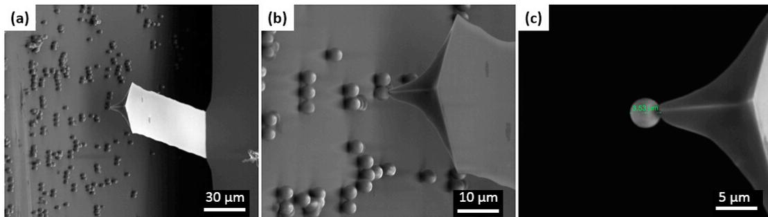
Fig. 2 - (a) SEM micrographs showing (a) the PMMA-coated beads dispersed on the silicon wafer, (b) contact of the AFM tip to one PMMA-coated bead and (c) an individual PMMA-coated bead attached to the apex of the AFM tip. The dimension of the bead was confirmed as 3.53 μm.
