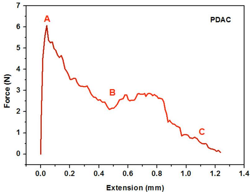
Fig. 7 - Typical force-extension curve recorded during the tensile separation of two PMMA surfaces bound by PDAC.
