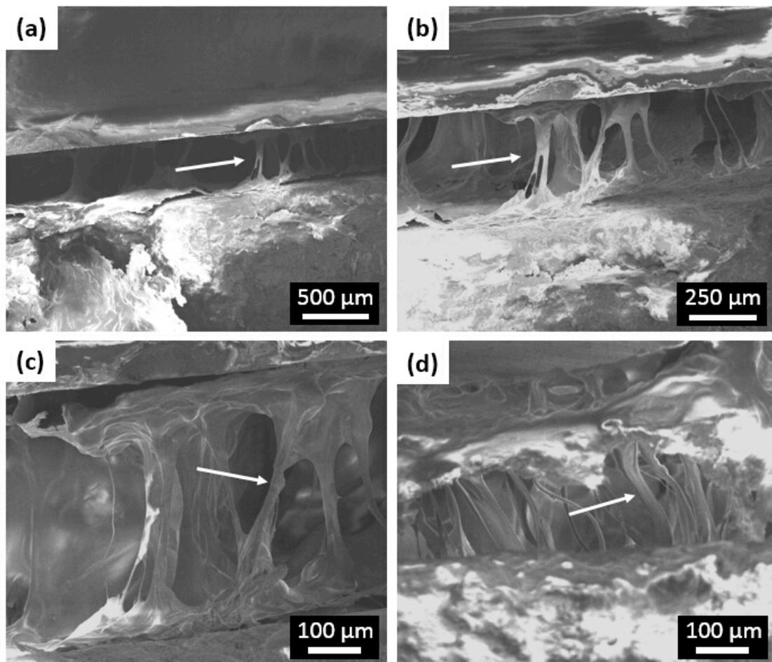
Fig. 5 - Scanning electron micrographs of the PDFP-bonded interfacial failure at higher sample strains. The images are obtained show the deformation behaviour of the
