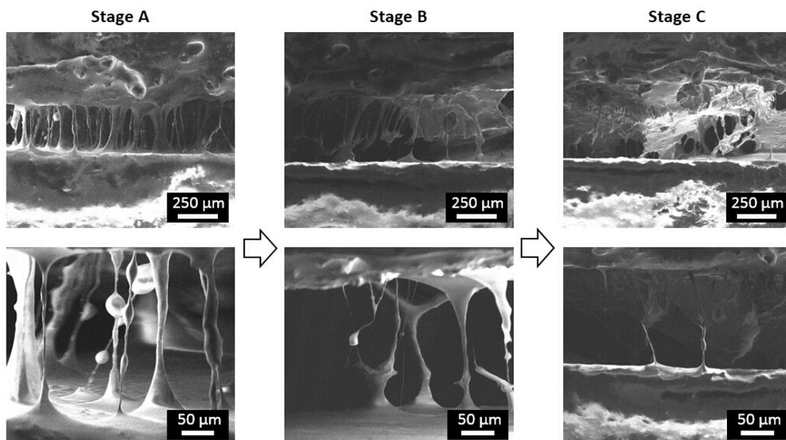
Fig. 8 - SEM micrographs at low ( $\times 200$ , top row) and high ( $\times 800$ , bottom row) magnifications showing the failure behaviour of the PDAC adhesive at stage A, B and C of Fig. 7.
