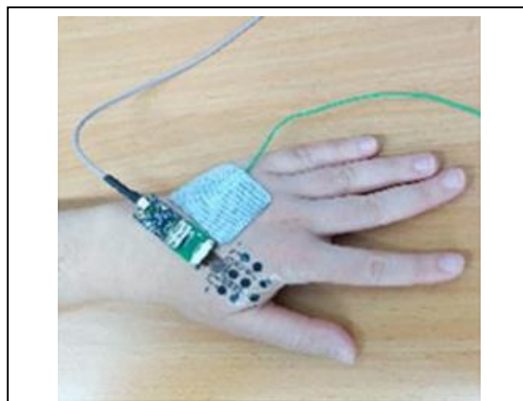
Figure 4. Electric tattoo consisting of a carbon electrode, an adhesive surface that sticks temporary tattoos to the skin and a nanotechnology-based conductive polymer coating, with special nanotopography, that enhances the electrode's performance.
