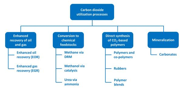
Figure 6. Carbon dioxide utilization processes, adapted from Al-Mamoori et al. [49].
