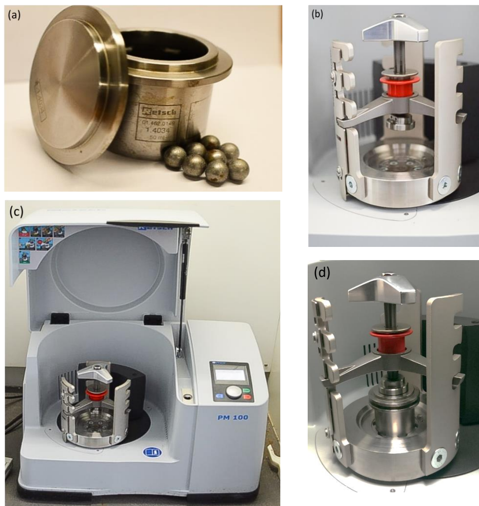
Figure 3-3: High-speed planetary milling equipment used with a) stainless steel grinding pot and balls; b) fixture for stainless steel pot; c) the complete device with programmable settings and d) stainless steel pot locked.
