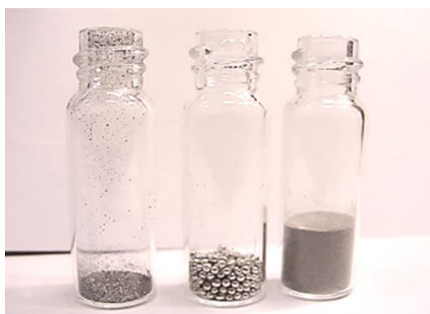
Figure 4-6: Particle size change with milling with and without additives. From right to left: aluminium powder non-milled, milled no-additives aluminium and aluminium powder milled with additives (metal oxide and salt).
