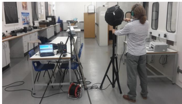
Figure 1 Example of a modern excitation system, including amplifier, dodecahedron loudspeaker, sound level meter (or microphone) and computer measurement platform.
