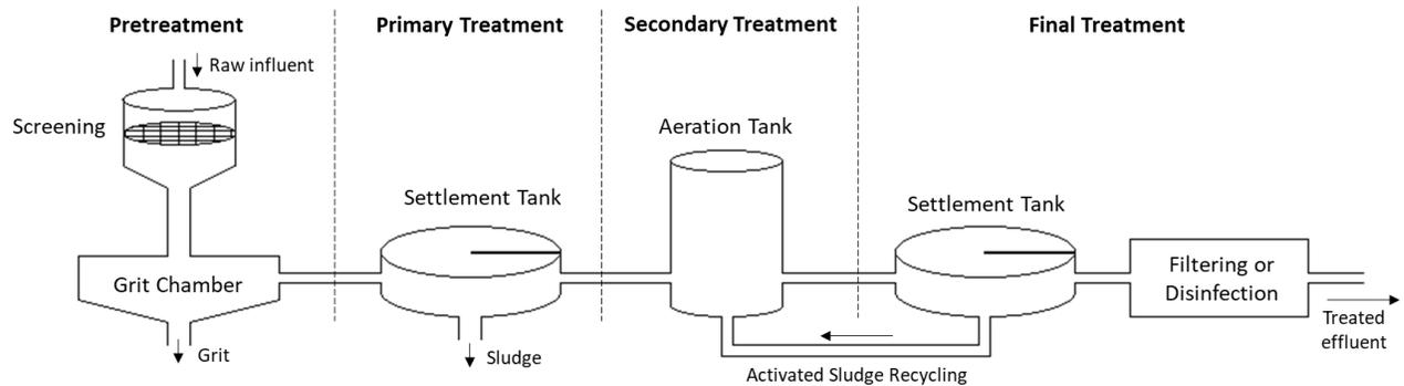
**Figure 2.** Representation of a typical wastewater treatment process.
