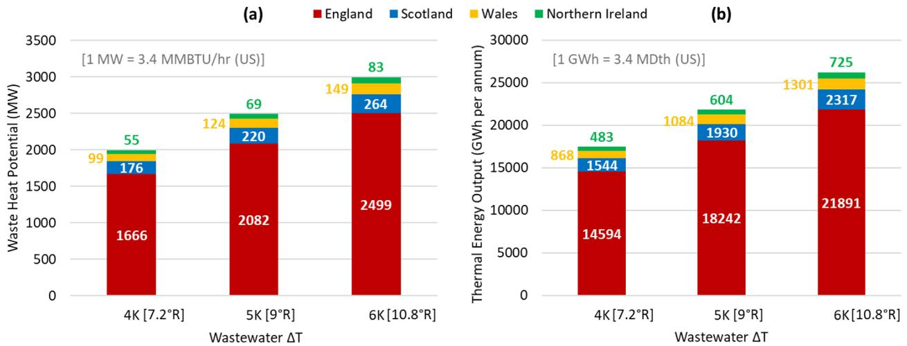
**Figure 3.** Theoretical values of waste heat potential (a) and annual thermal energy output (b) from WWTPs.
