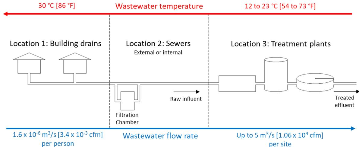
**Figure 1.** Locations for heat recovery from wastewater, with indicative flow rates and temperature for London.
