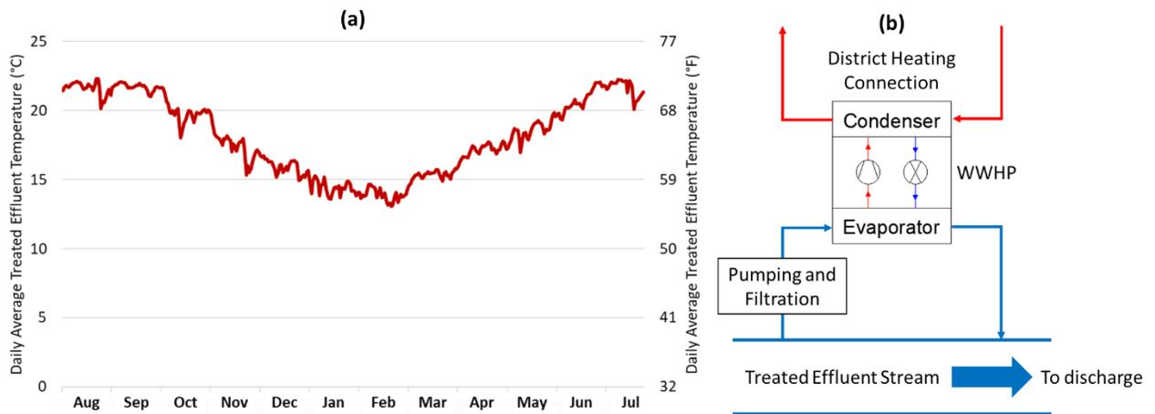
**Figure 5.** Temperature profile (a) and schematic of a heat recovery system (b) for the treated effluent from the Hogsmill WWTP.
