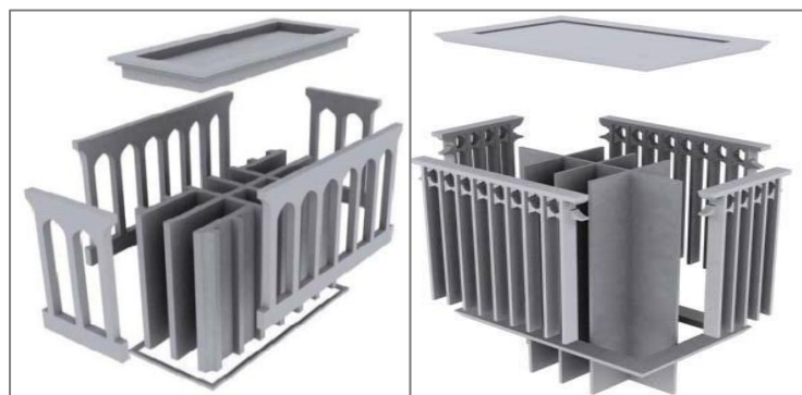
Figure 18: Wind catcher with different canals (Left) Equal canals (Right)
