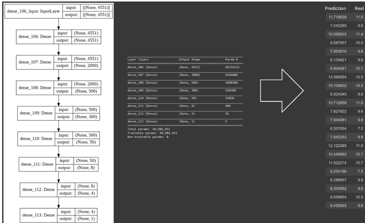
Figure 7.2. The structure of the neural network model designed for training with the spectral approach.
