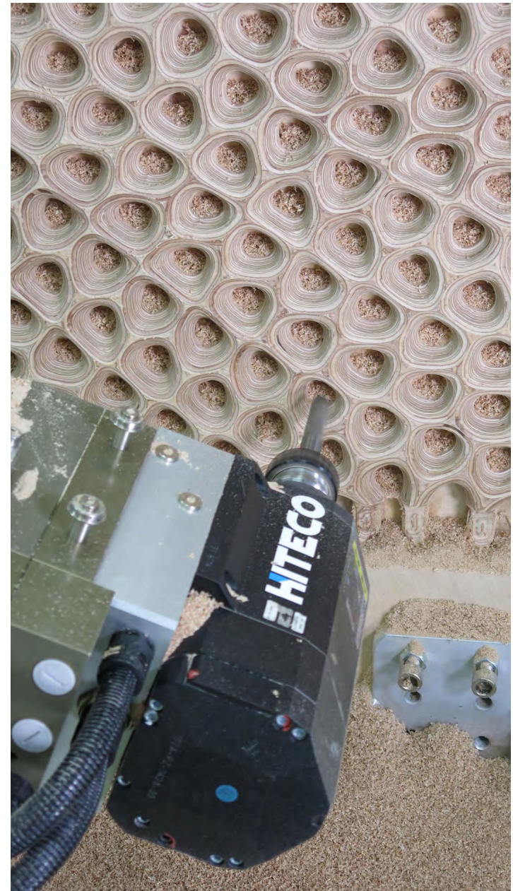
-FABRICATION PROCESS- / Morphogenetic pattern, robot milling. //
