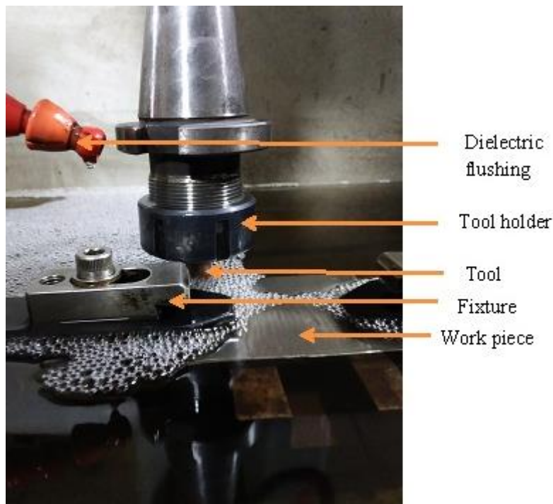
Fig. 1. A photographic view of the machining chamber of EDM experimental setup
