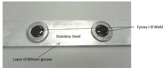
Fig. 4. A pair of a steel reinforced epoxy J-B Weld samples with a diameter 17 mm and thickness of 4 mm surrounded by a washer produced to measure thermal conductivity using a Hot Disk thermal constants analyser.
