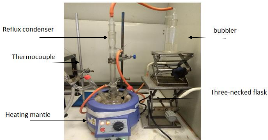
Figure 3. 4 Experimental set-up for the solution phase synthesis (organometallic reaction) of CoP.
