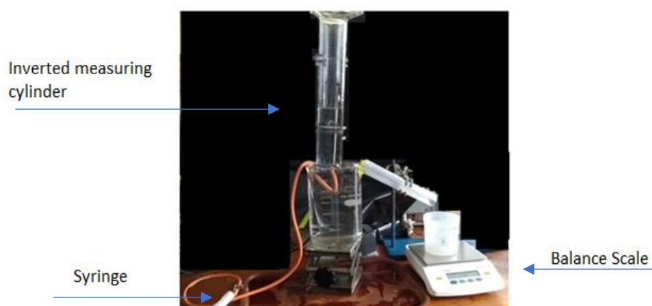
Figure 3. 15 Inverted column hydrogen collection set-up.
