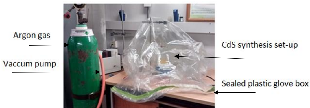
Figure 3. 1 Experimental set-up for the CdS synthesis in an inflatable glove box.
