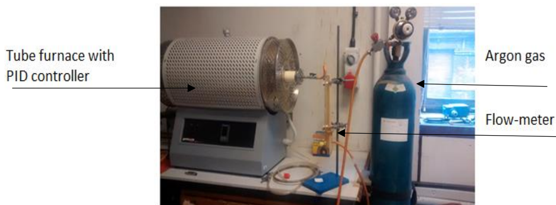
Figure 3. 3 Experimental set-up for the solution phase synthesis of \text{CoP} in an argon purging tube furnace with PID temperature controller.
