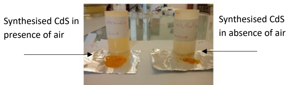
Figure 4. 1 Comparison of CdS powders prepared in air and in oxygen free environment.
