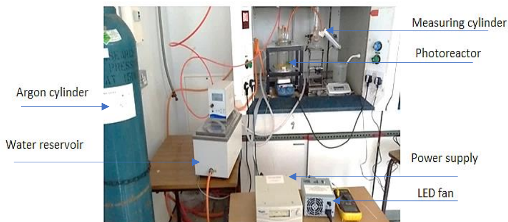
Figure 3. 16 The connected compartments for a typical photocatalytic hydrogen production.
