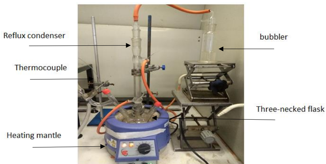
Figure 3. 2 Experimental set-up for the Pt synthesis under argon gas atmosphere.
