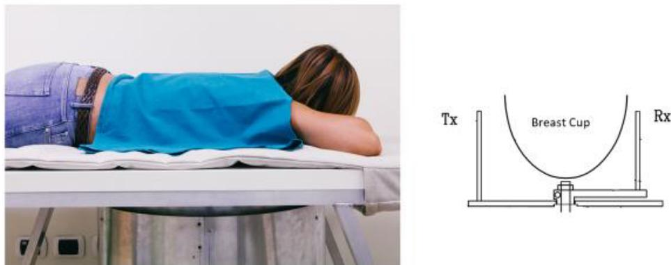
Figure 1. The microwave apparatus consists of a cup that holds the breast when the patient lies prone on the examination table. The transmitting (TX) and receiving (RX) antennas are located inside a hub and can be moved around the azimuth, to irradiate the breast (through TX) and capture the microwaves scattered by the breast itself (through RX).
