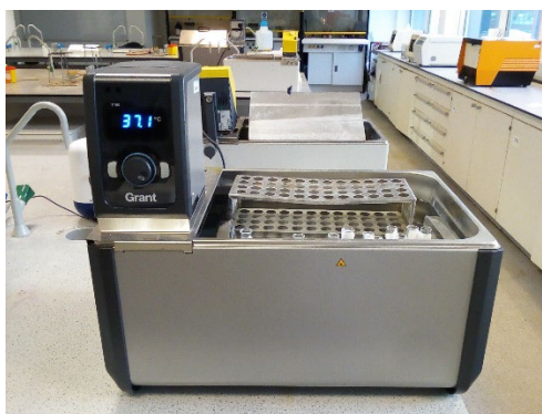
Figure 8.1. Test tubes being heated at approximately 37^\circ\text{C} to develop the blue-green colour for quantification of glucose.
