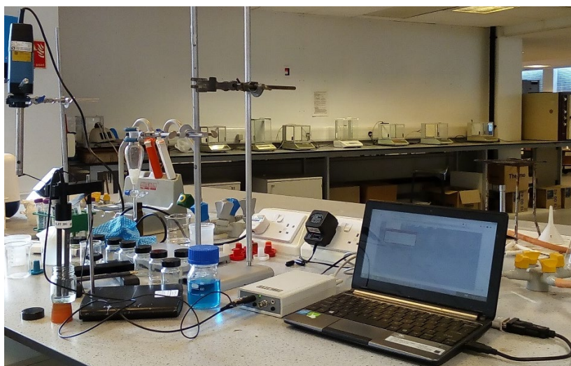
Figure 5.5. Reference and \text{NH}_4^+ ISE electrodes connected to the ELIT 801 pH/ISE Analyser and a Computer/ Data Recording System.
