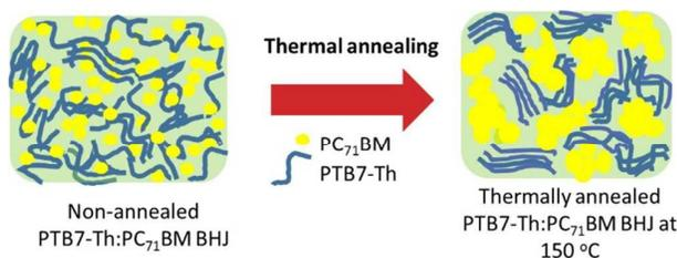
Figure 7: Schematic illustration of morphological changes happening to PTB7-Th:PC<sub>71</sub>BM blend films on thermal annealing.
