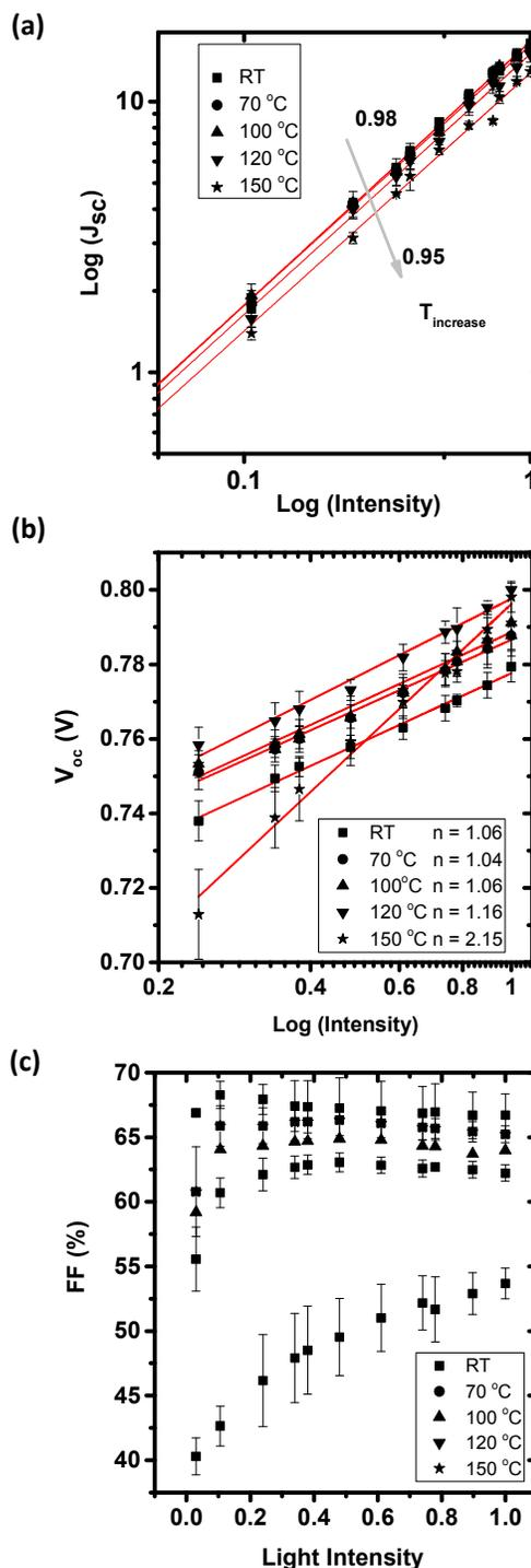
Figure 2. (a) J<sub>sc</sub> vs Light intensity, fitted to a power law relationship (b) V<sub>oc</sub> vs Light intensity (c) FF vs Light intensity of the PTB7-Th:PC<sub>71</sub>BM solar cell devices as a function of thermal annealing.
