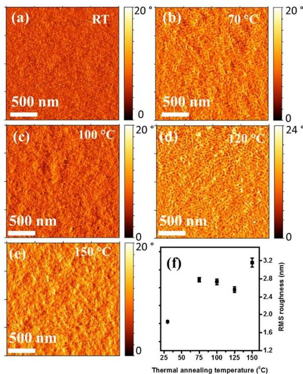
Figure 3. (a)-(e): Atomic force microscopy phase images of the PTB7-Th:PC<sub>71</sub>BM blends as a function of thermal annealing (f) RMS surface roughness as a function of thermal annealing temperatures.
