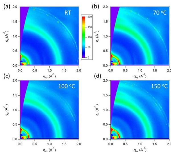
Figure 5. (a)-(d): GIWAXS 2D patterns of the PTB7-Th:PC<sub>71</sub>BM blend films as a function of thermal annealing.
