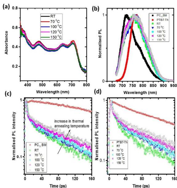
Figure 4. (a) UV-Vis absorption spectra and (b) normalised PL spectra of PTB7-Th:PC<sub>71</sub>BM blend films as a function of thermal annealing; (c) time resolved PL of the blend detected between 670 nm and 720 nm, which is dominated by emission from fullerene;
