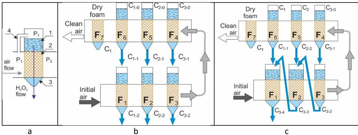
468 Figure 8. Principle scheme of the air filtration system: a) filter unit scheme consisting of 1
