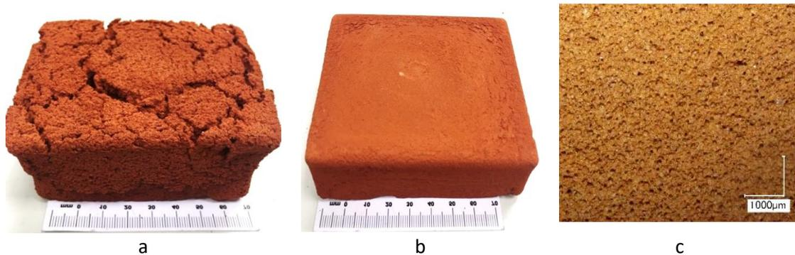
405 Figure 3. Foamed clay ceramic samples after sintering at 950 °C: a) WG0-950 (without
