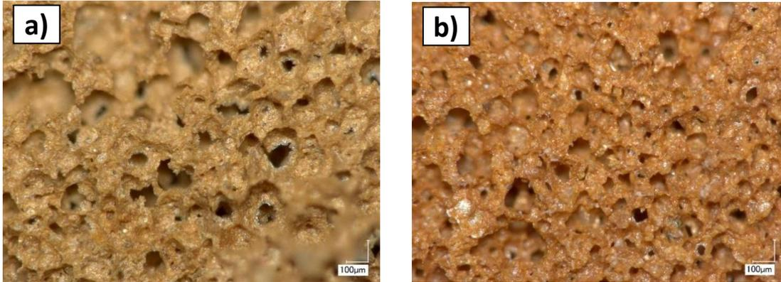
419 Figure 5. The optical microscopy images of glass containing foamed clay ceramic materials
