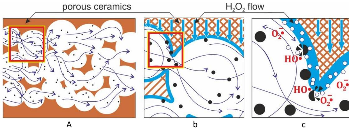
505 Figure 9. The contaminated gas motion in porous structure (a) acceleration and collisions
