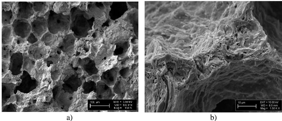
409 Figure 4. SEM images of fractured foamed clay ceramic sample WG5-950: a) general pore
