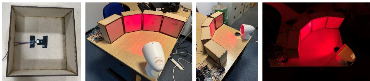
Figure 30 Testing the PDLC performance against Infrared light with light and temperature sensor
