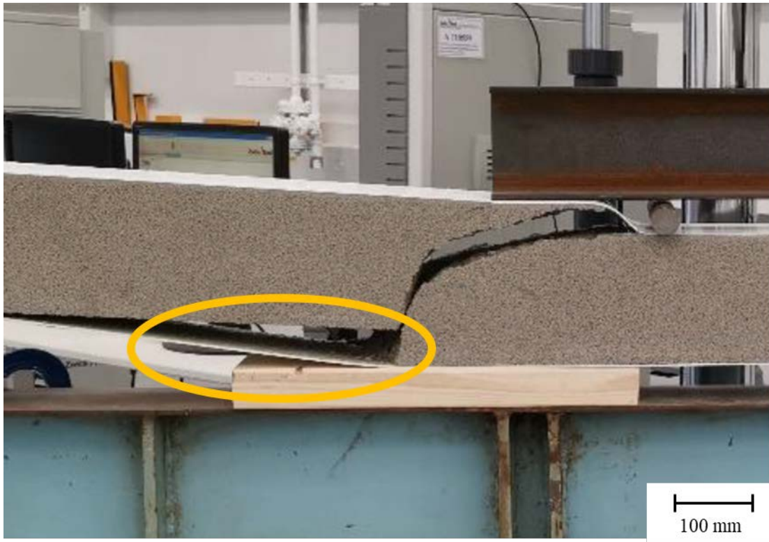
Figure 17: Failure mode observed in specimen P22-1-B150-L2250-XB showing tension side delamination of the facing sheet from the bead core.
