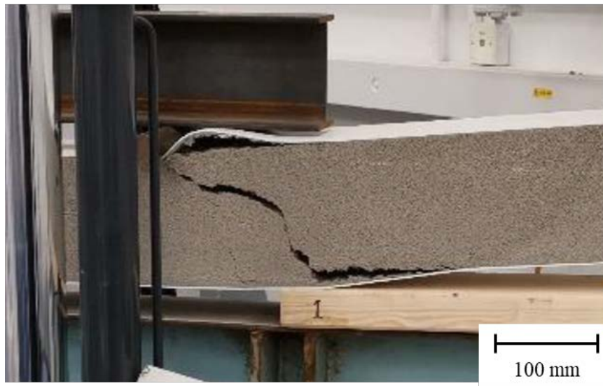
Figure 15: Typical failure modes exhibited in RGBSPs, with longitudinal cracking through a layer of bead core above the adhesive in conjunction with a diagonal shear-induced crack.
